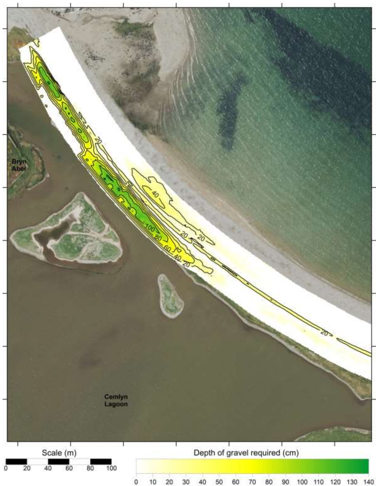
Figure 64. Enlargement of the NW section of the Cemlyn Barrier showing the depth of gravel required (in cm) to raise and widen the barrier to that shown in Figure 62.
