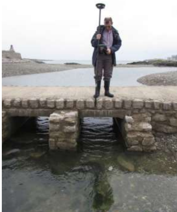
Figure 26. Surveying the elevation of the footbridge using Leica GNSS RTK GPS equipment
