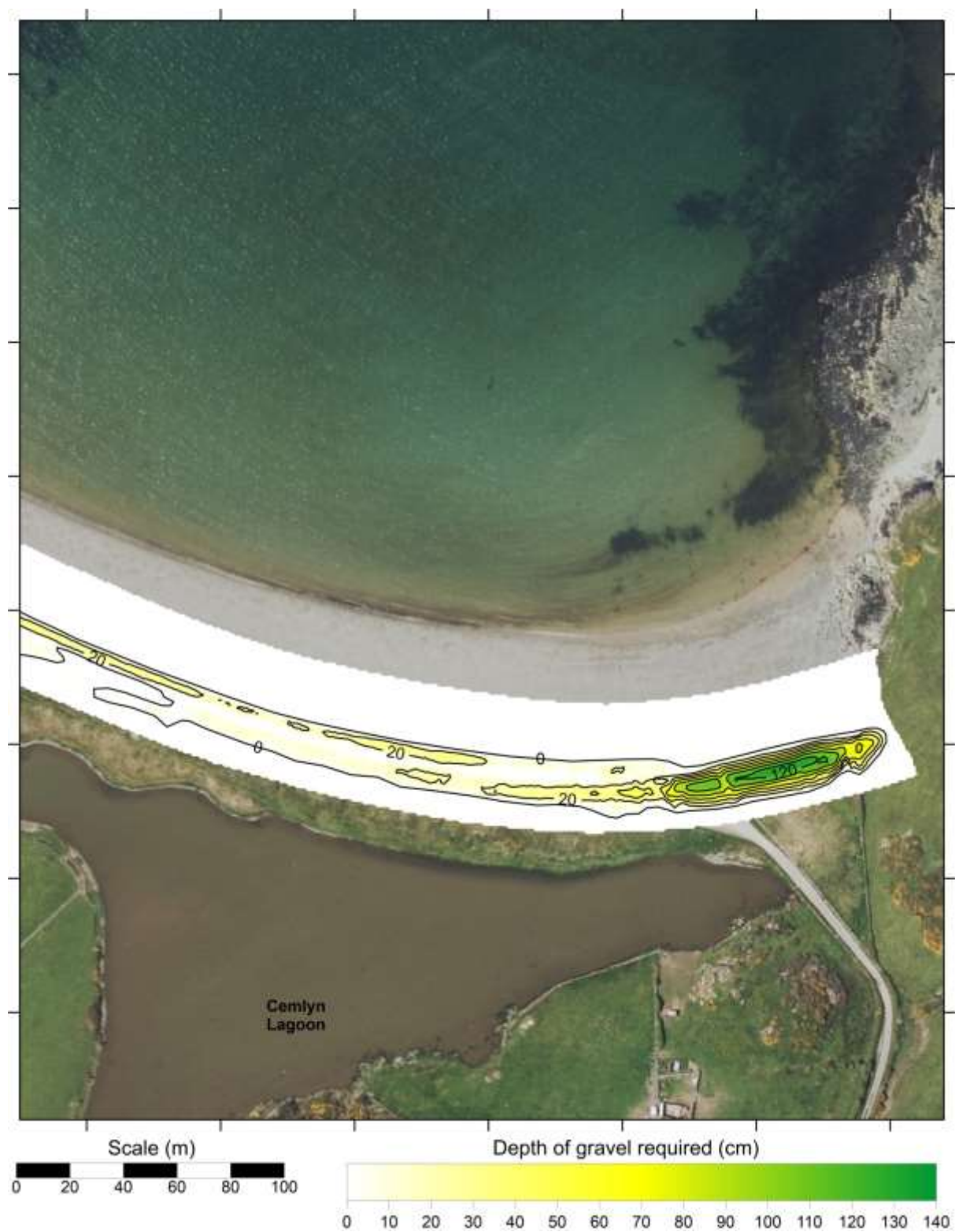
Figure 66. Enlargement of the SE section of the Cemlyn Barrier showing the depth of gravel required (in cm) to raise and widen the barrier to that shown in Figure 21.
